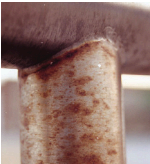
Severe tea staining of stainless steel in a coastal environment shortly after installation.
