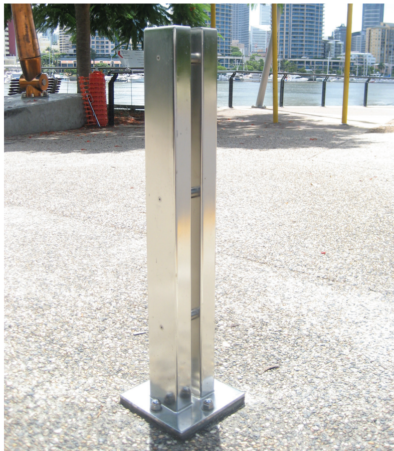
Electropolished stainless steel grade 316 in perfect condition after seven years of exposure in a marine environment.
