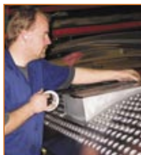
This photograph was taken a month after installation. Corrosion resulting from rough finishing technique is evident. Note also the crevices that are likely corrosion sites.
