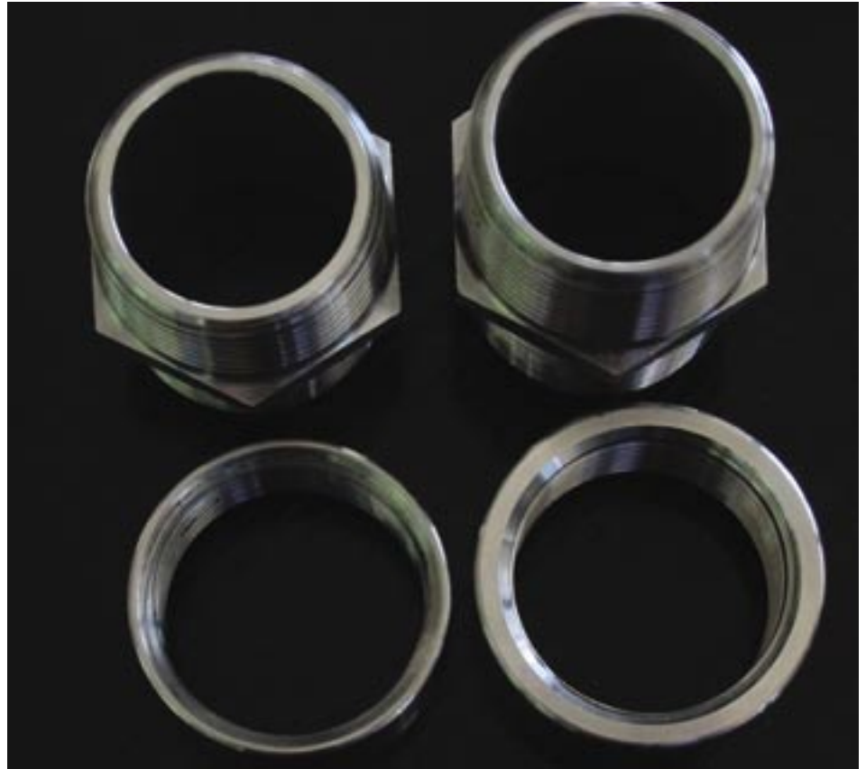
Above: the wall thicknesses of old (left) and new (right) threaded fittings
