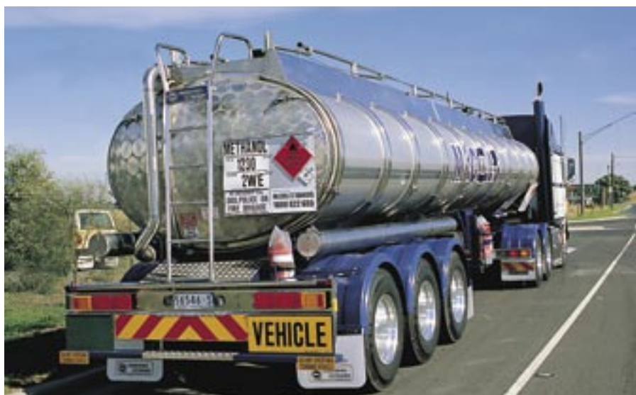
McColl's Transport carts a variety of chemicals such as caustic soda and formaldehyde. The tanker barrel has been wrapped and not rolled, with full length stainless sheets used to eliminate circumferential welds.
